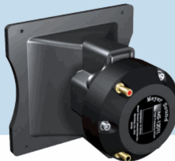
A single 3-inch diaphragm, 1.2-inch exit, neodymium magnet compression driver is mounted on Meyer Sound's patented REM manifold.
